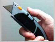
Slide the blade-advance button forward to use new blade.
