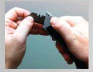
Press the button to release used blade.
