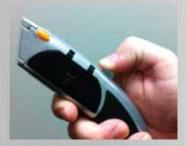
Slide the blade-advance button completely backward to refill new blade.
