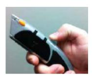
Slide the blade-advance button completely backward to refill new blade.
